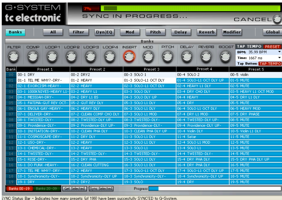
SYNC Status Bar - Indicates how many presets (of 199) have been successfully SYNC'ED to G-System.
